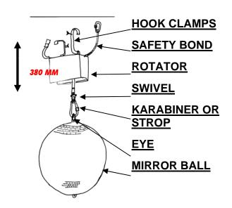
THE COMPLETE ASSEMBLY IS TESTED UNDER LOLER REGULATIONS.
